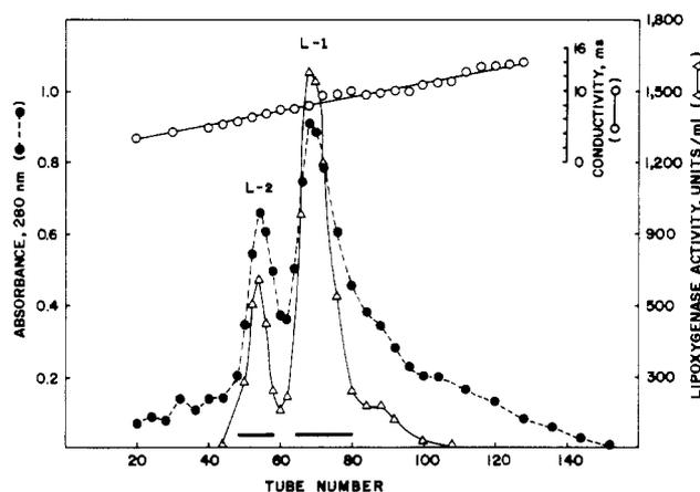
Figure 1. Separation of cowpea lipoxigenase isoenzymes on the DEAE-Sephadex A-50 column (2.5 × 30 cm). Five-milliliter fractions were collected at the rate of 32 mL/h by using Tris-HCl buffer, pH 8.0, with a NaCl linear gradient of 0.05-0.35 M.
