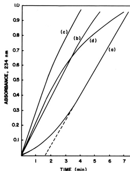
**Figure 4.** Progress curves of the oxidation of linoleic acid catalyzed by cowpea L-1 and L-2. (a and b) L-1 and L-2 with new linoleic acid solution; respectively; (c and d) L-1 and L-2 with old linoleic acid solution, respectively.
