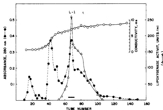
Figure 2. Hydroxylapatite column chromatography of DEAE-Sephadex A-50 pooled fractions. Column size: 2.2 × 18 cm. Three-milliliter fractions were collected by using a linear gradient of 0.01-0.3 M phosphate buffer, pH 6.8, at the rate of 8 mL/h.
