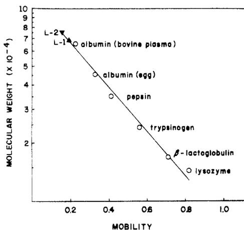
**Figure 5.** Calibration curve for determination of the molecular weight of cowpea L-1 and L-2 using NaDodSO<sub>4</sub>-polyacrylamide gel electrophoresis.
